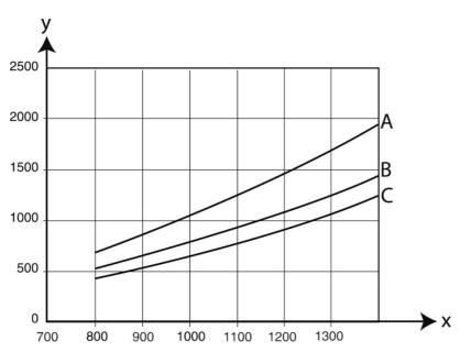
X: airflow, m<sup>3</sup>/h, Y: static pressure Pa,
