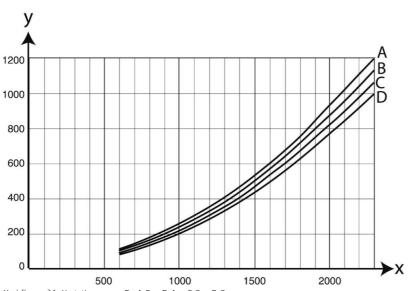
X: airflow, m³/h, Y: static pressure Pa, A: 5 m, B: 4 m, C: 3 m, D: 2 m  $\,$
