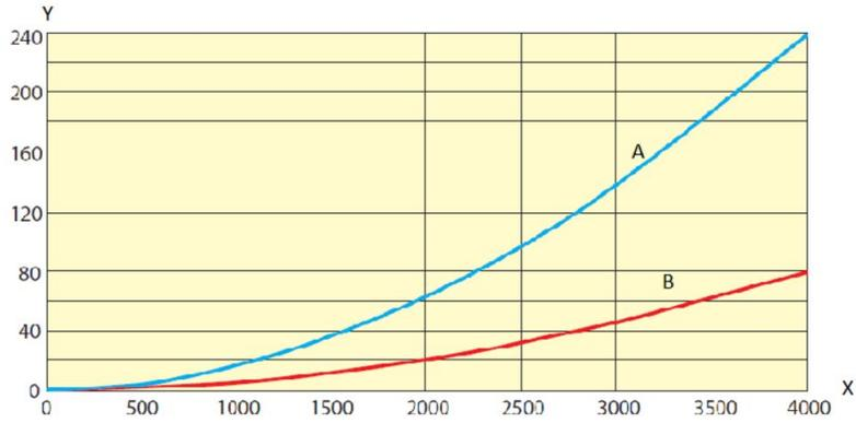
Y= Pressure drop (Pa), X= air flow (m<sup>3</sup>/h)
