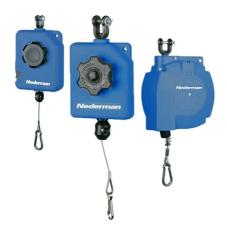
Series 810 balancer makes the tool weightless and minimizes the strain on the operator. The balancer comes in three different models and in nine weight classes, with a span from  $0.5 \, \text{kg}$  to  $10.9 \, \text{kg}$  (1 lb to  $24 \, \text{lb}$ ).
