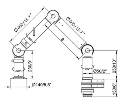
EK 2000 Arm(s): 1 x FX2 50 arm Hood(s): 1 x combination hood Hose: Ø 75 mm (3 inch), 3000 mm (118 inch) length Max. airflow: 100 m3/h (58.8 cfm)
