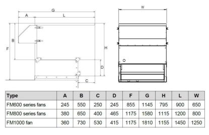
DUAL-Silencer dimensions (mm) with air grille and rain cover (for outdoor use)
