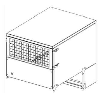
The DUAL—silencer encloses the fan motor and the top of the fan case. It may be fitted to any FM unit and take the place of a conventional in–line silencer, with the added benefit of reducing breakout noise from the fan.
