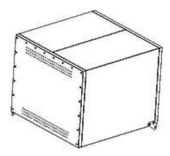
Both side panels with cooling air openings are de-mountable for access to the fan motor.
