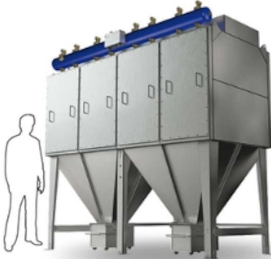
The FMK25 range is a reverse jet cassette dust collector. It was built for continuous use in industrial process filtration and dust collection applications. The FMK dust collector uses our long established fabric pocket cassette that is easily maintained through the front hinged doors. The cassette offers ample filter area and lasts longer than a cartridge.
