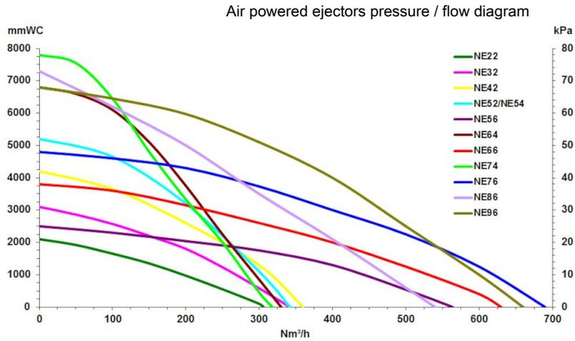
Air Powered ejectors
