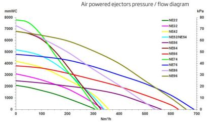
Air Powered ejectors
