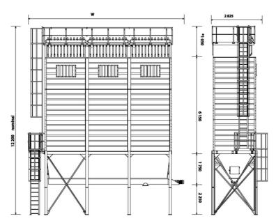
Hopper heights are typical values for  $55^{\circ}$  valley angle trough hopper
