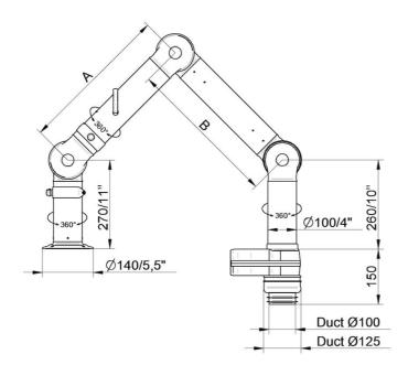
• FX2-ESD/EX-D100-L1200-Up/Down-Low Part number: 70606544 Max. rayon d'action: 1170 mm (46,1 in) A: 450 mm (17,7 in) B: 450 mm (17,7 in)
