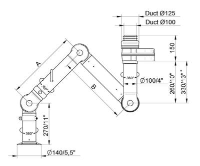
• FX2-ESD/EX-D100-L1200-Up/Down-Low Part number: 70606544 Max. rayon d'action: 1170 mm (46,1 in) A: 450 mm (17,7 in) B: 450 mm (17,7 in)
