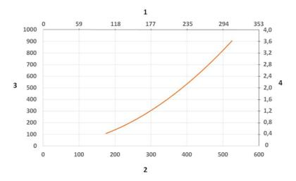
Pressure Drop diagram: 1) X- Axis: Air Flow Rate (cfm) 2) X- Axis: Air Flow Rate (m/h)
