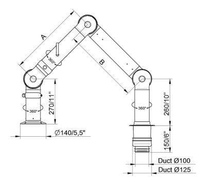
• FX2-ESD/EX-D100-L1200-Up/Down-Thru Part number: 70606744 Max. rayon d'action: 1170 mm (46,1 in) A: 450 mm (17,7 in) B: 450 mm (17,7 in)
