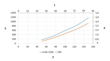
Pressure Drop diagram: 1) X- Axis: Air Flow Rate (cfm) 2) X- Axis: Air Flow Rate (m/h)
