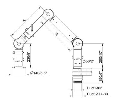
• FX2-ORIG-D50-L700-Up/Down-Low Part number: 70600144 Max. working radius: 630 mm (24,8 in) A: 400 mm (15,7 in) R: -
