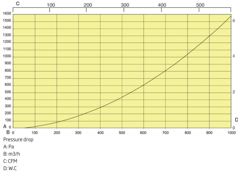
Pressure drop valid for 6 and 7 m track with 5 m hose, Ø 125 mm, and HB 600LL nozzle.
