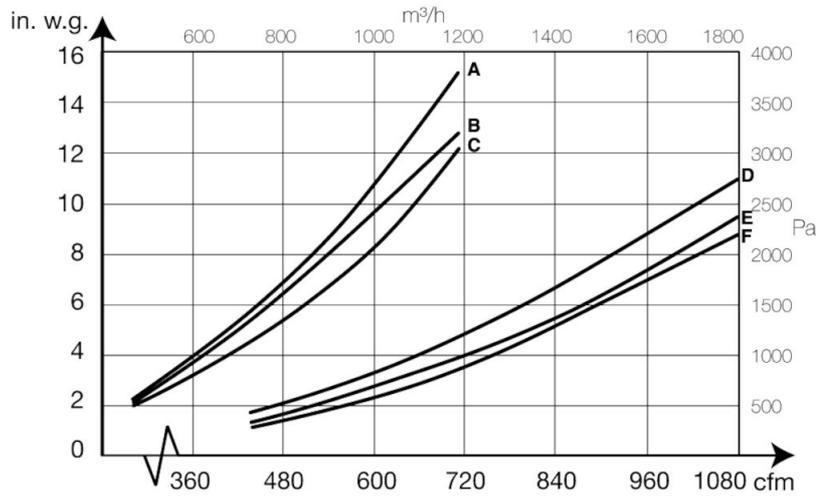
X: airflow m³/h Y: static pressure Pa A= 4 m Ø125 mm, B= 3 m Ø125 mm, C= 2 m
