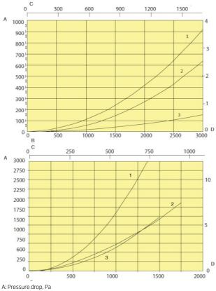
B: Airflow, m3/h C: Airflow cfm D: Pressure drop, in w.g.
