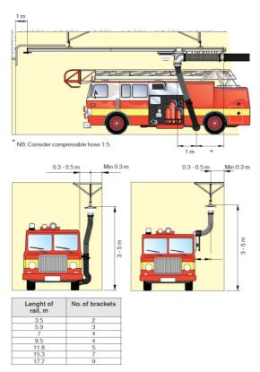
N.B. The nozzle for high level (HL) exhaust pipes must be installed at a higher level than the exhaust pipe. The nozzle must be pulled downwards at connection, which will activate the balancer.
