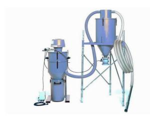
This robust and extremely powerful system is designed for the recovery of blasting shot. Equipped with automatic pneumatic pinch valve and automatic self-cleaning NCF filter. Most of the dust is separated from the blasting shot or from the collected granulates. The dust is channelled into its own container, while the blasting shot or granulated material is fed back into the blasting pot, onto conveyors or into other containers.
