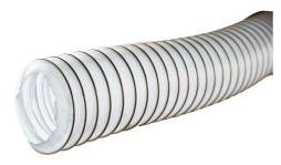
Very flexible hose, light weight. Suitable for transporting abrasive material such as wood shavings, sawdust, cement dust, granulates and technical gases in the chemical and petrochemical industries. Very good resistance to wear and ageing. Good resistance to fuels, oils, solvents and grease.
