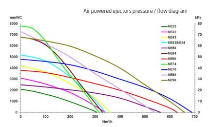
Air Powered ejectors
