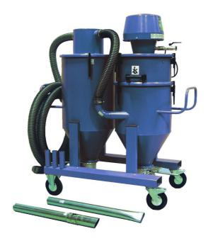
Powerful and flexible industrial vacuum cleaner unit installed on trolley, equipped with a grit/dust discharge unit on pre-separator silo. The cleaned grit can be emptied into a bucket, feed system or floor bin. The dust is trapped in the NCF filter and collected in the second stage silo. Suitable for use in blasting halls for grit recovery and cleaning of blasted hulls and steel structures.
