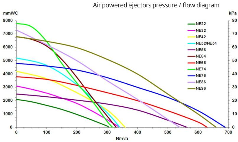
Air Powered ejectors
