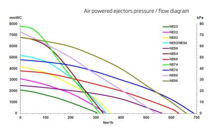
Air Powered ejectors
