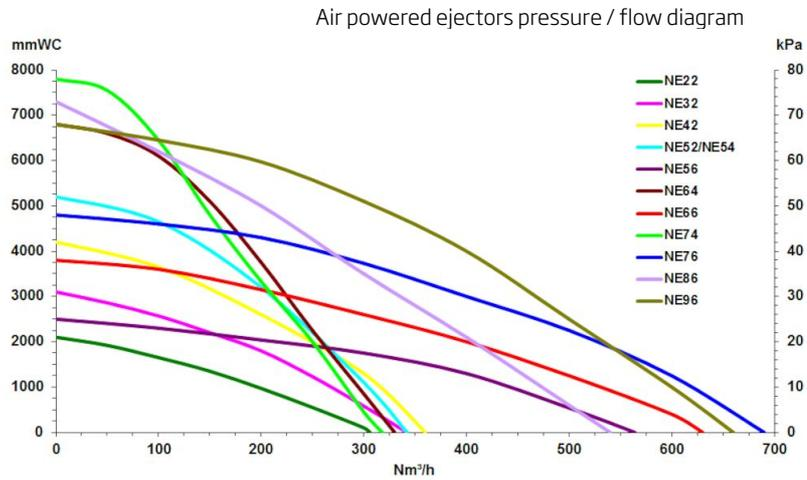
Air Powered ejectors
