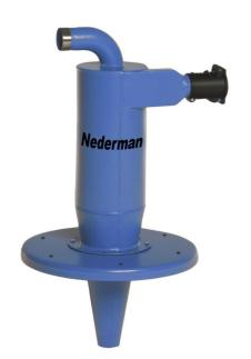
Cyclones are normally used when a maximum pre-separation of collected material from the transportation airflow is required. Cyclones are normally located on silos, tanks, containers etc. suitable to store the collected material and thereby functtion as a deead chamber under the cyclone. Normally, a filter stage shall be installed between the cyclone and the vacuum power unit.
