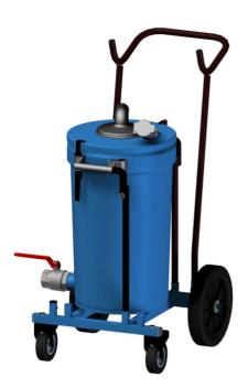
Mobile pre-separator for collecting and recycling of oil, cutting fluid, coolant, water and other non-flammable liquids. Perfect formachining and process industries, drilling, milling and turning. A float ball automatically shut off the suction flow when the container is full. The mobile pre-separator is equipped with a tippable container for easy discharge of collected liquids. The inlet and outlet diameter is 51 mm (2 in) for coupler (43930101 and 43930102).
