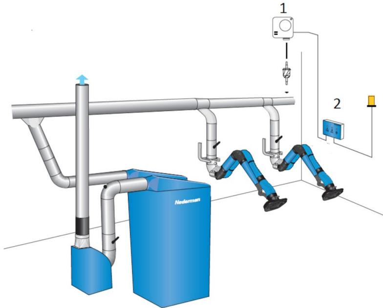
Airflow alarm and pressure switch mounted
