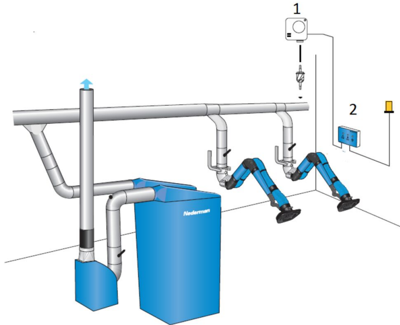
Airflow alarm and pressure switch mounted
