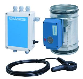
The motor damper consists of an operation box that can be controlled by a contactor or switch. The operation box consists of a 30 VA transformer for the lighting kit in the extraction arm, a delay timer for fan stop variable from 0-5 minutes, and two separate connections for sensor clamps.
