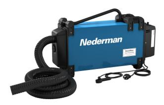
The Fume Eliminator 860 is designed to be carried to the working area. Although it can be used with a nozzle, it is specifically developed for on-torch applications - connected directly to the welding torch, it extracts the fume directly at the source. The FE 860 has a knob to set the desired suction level, an automatic start/stop function, which starts the unit as soon as the welding begins and significantly improved motor performance (versus the FE840/841).
