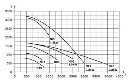
X: airflow, m³/h Y: static pressure Pa
