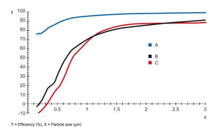
A = NOM filter, B = Centrifugal filter A, C = Centrifugal filter B
