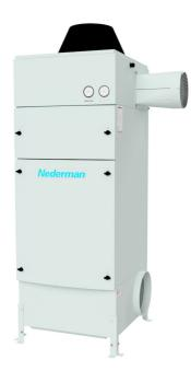
Designed for lathing and milling applications, for machines stamping and pressing steel plates, industrial washing machines, abrasive water jets etc. In all metal fabrication with oil mist troubles, these filters will fit into a ducting system, connected to each machine. All units are equipped with pressure gauge for control of filters as well as an indication for need of cleaning (self draining). Suitable for emulsion mist.
