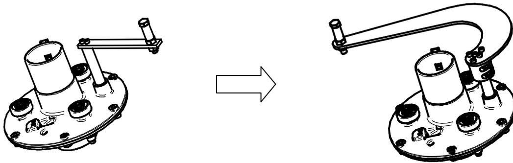
1. Replace the old damper housing with the new.
