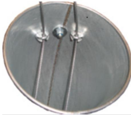
The release of the magnet is achieved by means of two wires inside the vertical hose. One wire is attached to the back of the magnet inside the magnet assembly, and the other wire is attached to a spring inside the magnet assembly. The other ends of the two wires are attached inside the elbow with the balancer, see the figure above.
