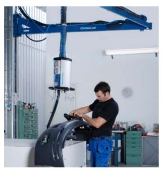
The flexible jointed arm makes it possible to reach several workspaces, and can easily be stowed away.
