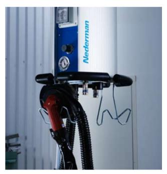
Cables and hoses are kept off the floor reducing the wear. Tools are easy accessible on the tools holders.
