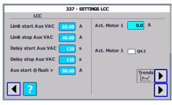
An auxiliary VAC unit will be started when VAC current load reaches "Limit start Aux VAC" and will stop once it decreases to "Limit stop Aux VAC". Starting and stopping of auxiliary units will be delayed by its corresponding delay setting.
