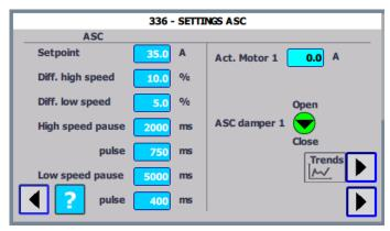
A VAC has a risk of "pumping" at low airflow, thus the airflow is kept, by false air, high enough to avoid this. The motor current is used as the control parameter.
