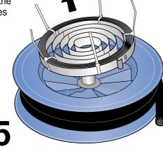
Remove the damaged spring.
