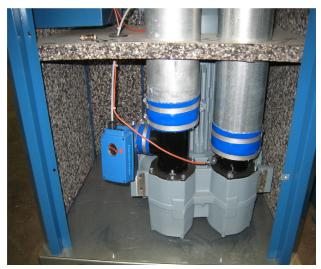
11). Depending on FlexPak manufactoring year, the vacuum valve cables, PT 100 cables and motor cable might be routed through the motor cover plate. Release all cables from the motor cover NOTE! Pay attention to how cables are routed
