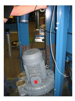
17) Carefully lift the blower out. Pay attention not to damage the vibration absorbers as they will be reused (NOTE! Blower weight: approx 130 Kg).
