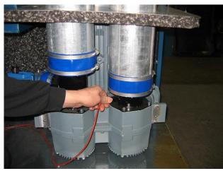
9) Unscrew the gland nut and remove the PT100 sensor rod. Be careful not to damage the sensor rod.
