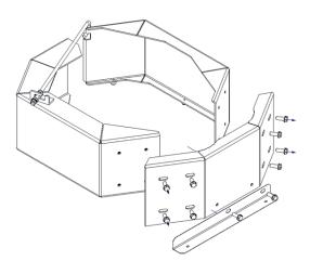
7) If the FlexPak is fitted with the FlexPAk upgrade kit, covering the blower, this has to be temporally removed in order to gain access to the blower.
