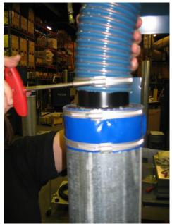
24) Refit the flexible hose to the top of the intake silencer.
