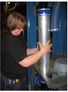
23) Refit the silencers and tighten the hose clamps.
