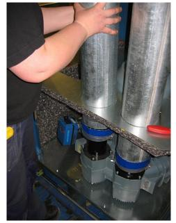
14) Remove the two silencers (up and out).
