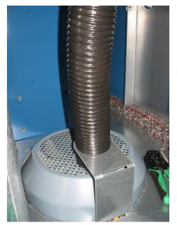
28) Fit the flexible hose to the bracket. Ensure that the hose is pushed flush against the motor grid/cover.
