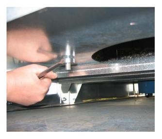
16) Unscrew the nuts securing the blower to the base. Access via the fork lift entry. NOTE! Base plate might have sharp edges. Use gloves and long sleeves.
