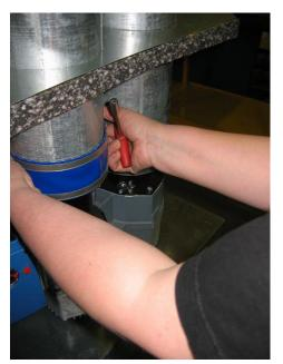
13) Remove the two upper hose clamps between the adapters and silencer pipes.
