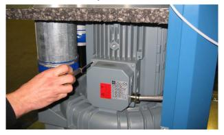
10) Disconnect the blower mains cable from the blower motor.
