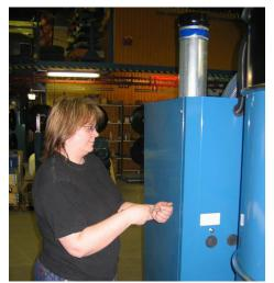
4) Remove the rear panel. Note! Unscrew the lower screw securing the panel to the base plate. Screw is located under the base plate and is accessed via the opening for the forklift.
