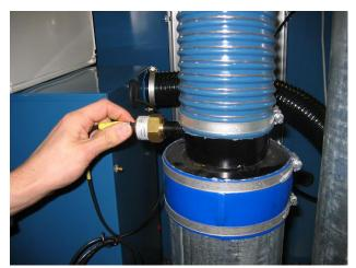
5) Disconnect the contact from the pressure transducer
