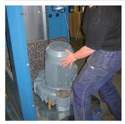
20) Fit the refurbished blower into position.
