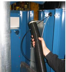
6) Remove the flexible hose between the motor and inverter housing
