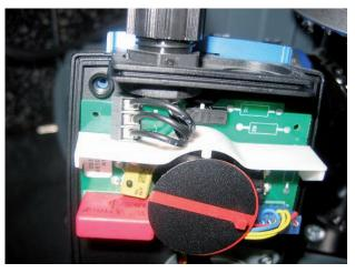
27) Refit the vacuum limit valve and connect wires to previous positions.
