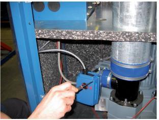
8) Remove the vacuum valve cover, and disconnect the wires. NOTE! Mark the position of the wires for correct re-assembly.
