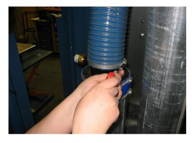
12). Loosen the hose clamp and disconnect the flexible hose from the inlet silencer.
